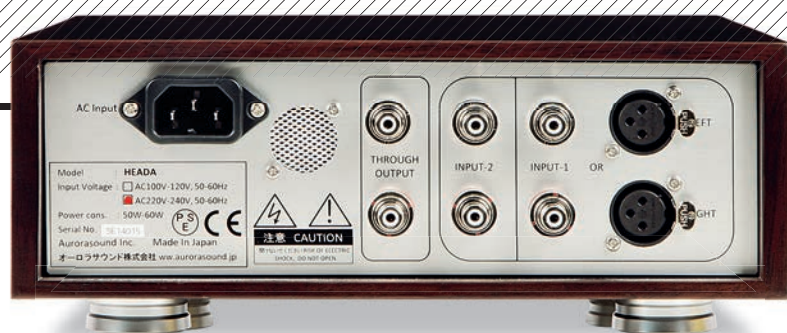
ABOVE: Input 1 offers balanced or unbalanced connections while Input 2 is unbalanced only. 'Through Output' bypasses the volume control, so the Heada cannot serve as a preamp with a separate power amp
